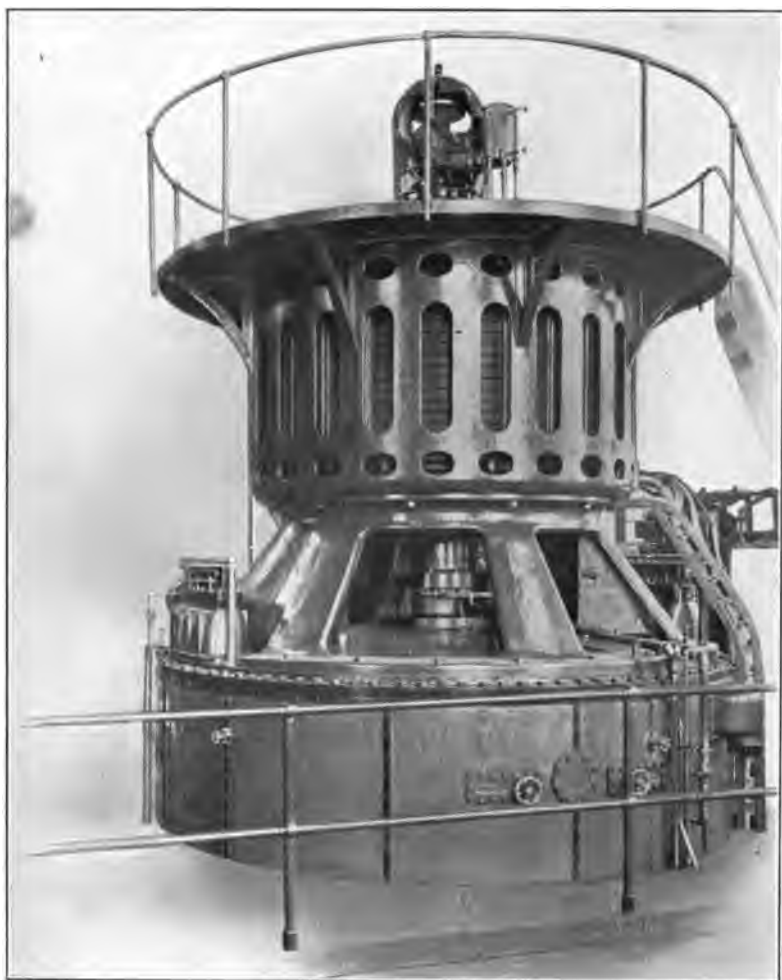
FIG. 285.—Outside View of a Curtis Turbine, Showing Generator at Top.
